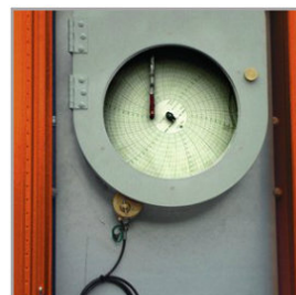
Recording instrument for tension meter
